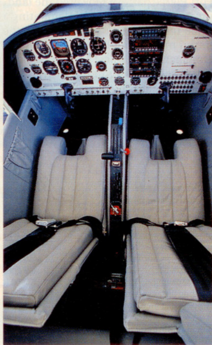
N223MJ is one of the last Miccos to be equipped with Bendix/King avionics (above). A stack of radio gear from UPS Aviation Technologies will replace it. The engine intake scoop (far right) is modeled after a Chevy Camaro's hood scoop.
